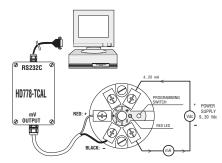
Instead of the thermocouple calibrator, you can use the Delta OHM HD778-TCAL: this instrument has to be connected to a serial port of the PC and, by means of a proper software, automates all the steps described below for programming the operating range.
